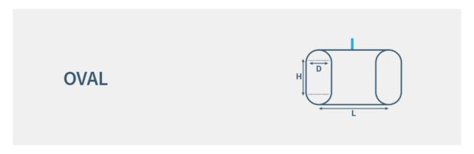
As described on the picture, the tank height must be calculated following this rule: total heigh – diameter.
