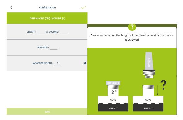
The adaptor is the tube length above the tank. It should not be longer then 7 cm otherwise the measurement could be false.
