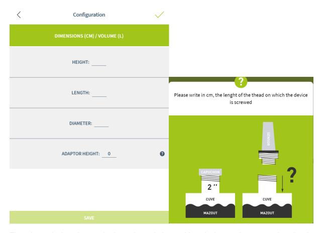
The adaptor is the tube length above the tank. It should not be longer then 7 cm otherwise the measurement could be false.
