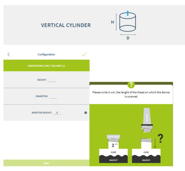
The adaptor is the tube length above the tank. It should not be longer then 7 cm otherwise the measurement could be false.
