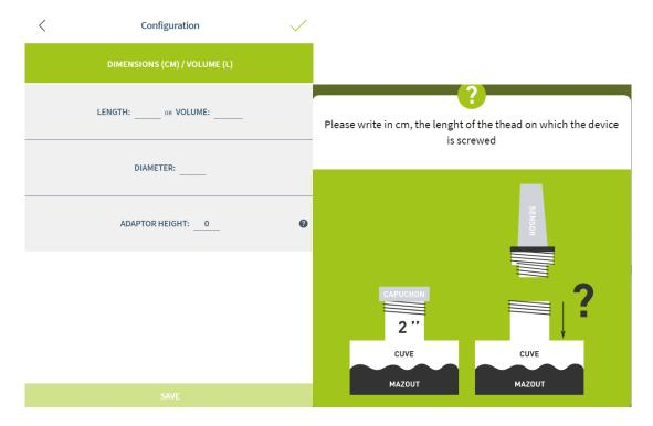
The adaptor is the tube length above the tank. It should not be longer then 7 cm otherwise the measurement could be false.
