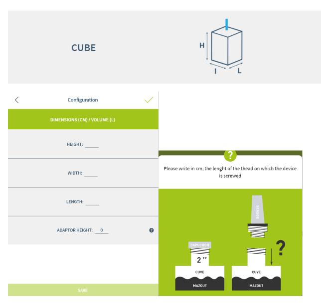
The adaptor is the tube length above the tank. It should not be longer then 7 cm otherwise the measurement could be false.
